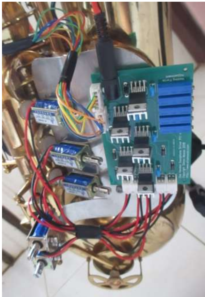
Fig. 6: Solenoid and driver assembly
