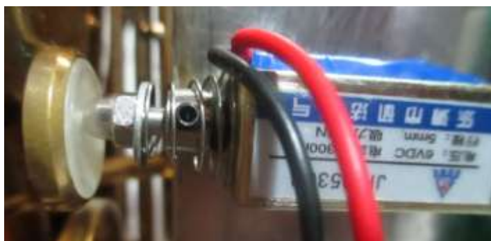
Fig. 13: Return spring used to assist solenoid activation and locking bush to prevent full retraction of the solenoid
