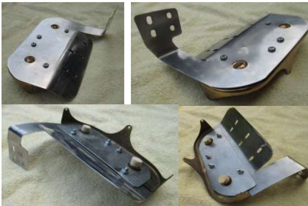
Fig. 5: Solenoid and driver circuit mounting bracket attached to guard cover
