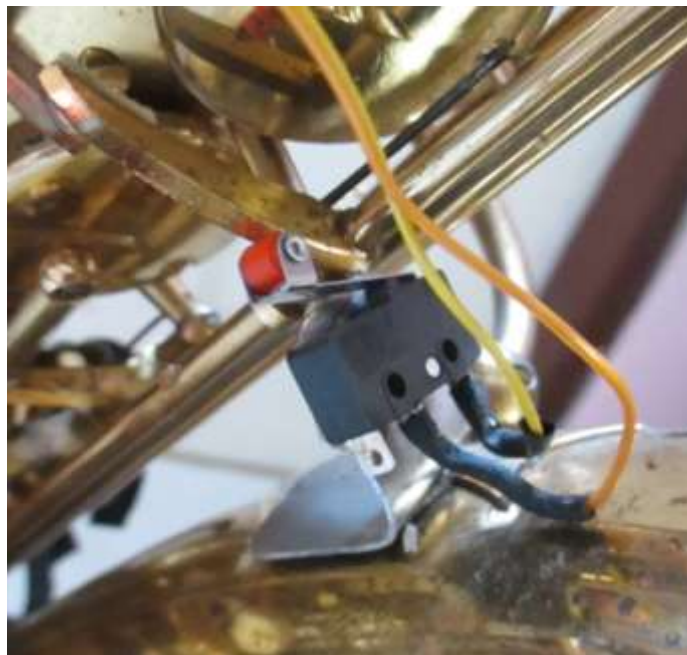
Fig 16: Location of the switch for lower C \sharp
